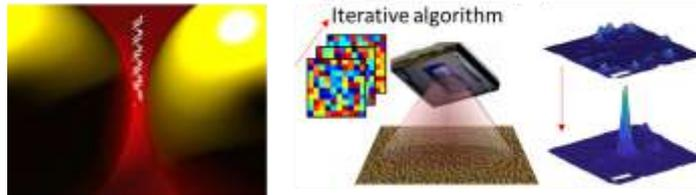
*Addressing plasmonic hot-spots: deterministic introduction of a controlled number of emitters using DNA-based self-assembly or far-field wavefront-based optimization in a disordered gold surface.*
