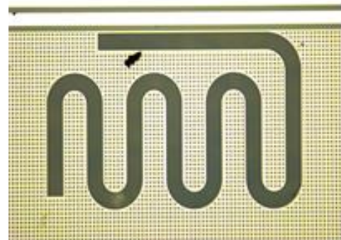
Superconducting Silicon resonator coupled to an Al transmission line and surrounded by an Al ground plane
