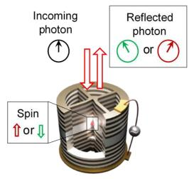
Principle of a spin-photon interface: the polarization of reflected photons is macroscopically rotated clockwise or counter-clockwise, depending on the embedded spin state
