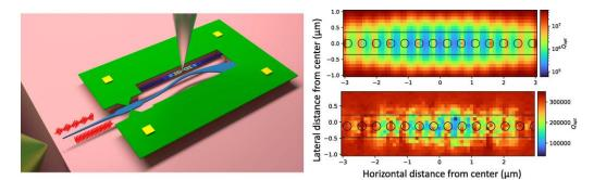
Left, Artist view of the measurement setup. Right, perturbations of the optical quality factor through the tip presence, with on top the simulation and on the bottom one measurement with a tip surface distance of 150 nm."
