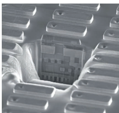
FIGURE Scanning Electron Microscopy image of a filamentary memristor in the back end of line of our hybrid memristor/CMOS process
